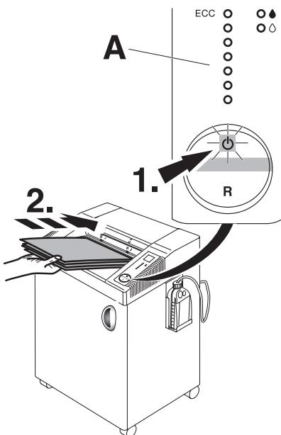
**EN** Press the rocker switch (1.) : green light is on, the machine is now ready for operation. Starts automatically when paper is inserted. Automatic standby that switches off after 1 hour. Green LED control light is off.
