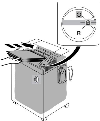
**EN** Stops automatically when plastic bag is full. Empty the bag when "bag full" indicator lights. (See page 8). Shake the container severral times to ensure a clean removal (1. ; 2.).
