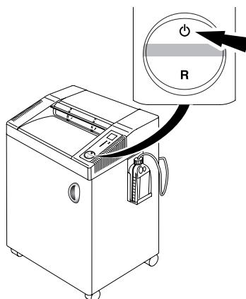
**EN** Automatic standby that switches off after 1 hour. Green LED control light is off.
