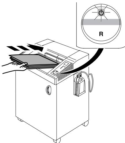
**EN** Stops automatically if too much paper is inserted. Automatic reverse if paper jams (Symbol "ON/OFF" ⏺ flashes).
