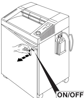
**EN** Remove the plug before cleaning the machine!
