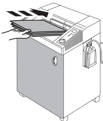
**EN** The door must be closed when operating the document shredder!
