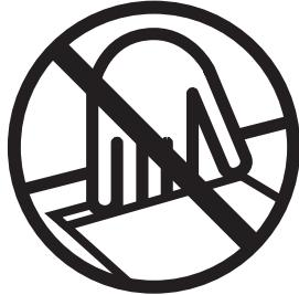
**EN** Do not reach into the feed-opening of the cutting head!
