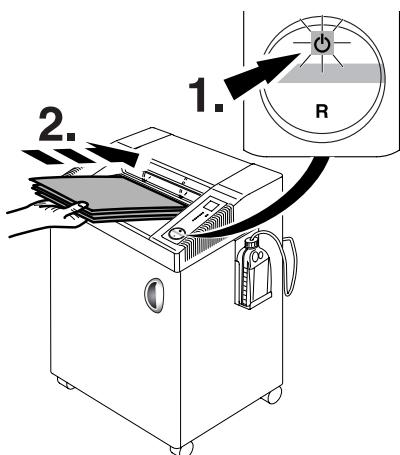
**EN** Reset by pressing the rocker switch  $\textcircled{R}$ .
