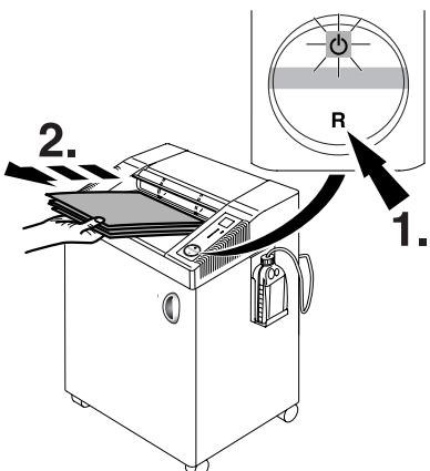
**EN If required:** Press the rocker switch "R" and remove paper. (Machine runs for a short time in reverse, if required repeat several times)
